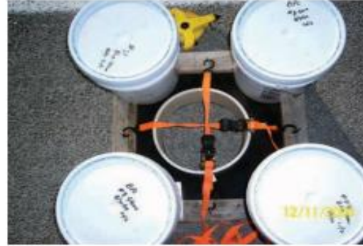
FIG. 4—Modified ASTM C1701 using neoprene seal on the porous surface at the U.S. EPA laboratories in Edison, NJ [10].
